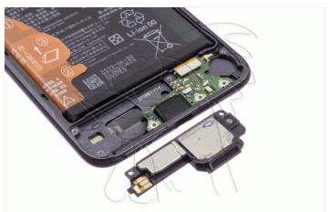
We disconnect the interconnection flex and the coaxial cable from the auxiliary plate, and using a flat tool we will detach the plate that we are going to replace.
