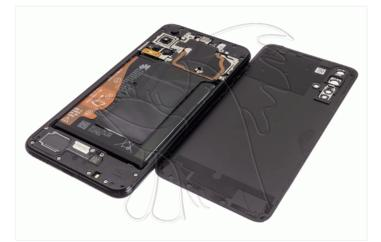
We remove the nineteen Phillips screws (PH # 00) that hold the intermediate housing, we will also use to remove the card tray, and with a thin tool we will unhook all the edges of the intermediate housing.
