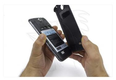
Remove the battery by pulling on the bottom.
