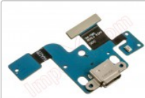
Auxiliary board with microphone, charging connector, data and accessories
