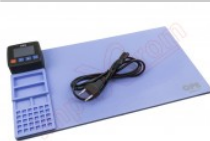
Heat-opening thermal mat, CPB320
