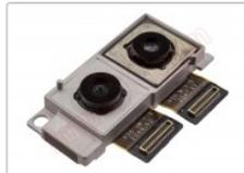
12.2Mpx and 16Mpx rear cameras module for Google Pixel 5, GD1YQ
