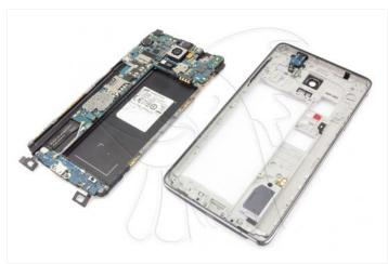
Step 9 - Removing the motherboard
