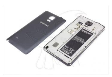
Finally, removing the battery will be as simple as lifting it with the help of a tool or with your hands.
