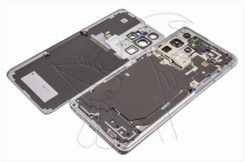
Step 2 - Shield with NFC antenna and wireless charging coil
